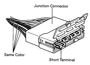
Junction connector (code: J1, J2, J3, J4, J5, J6, J7, J8, J9) in this manual include a short terminal which is connected to a number of wire harnesses. Always perform inspection with the short terminal installed. (When installing the wire harnesses, the harnesses can be connected to any position within the short terminal grouping. Accordingly, in other vehicles, the same position in the short terminal may be connected to a wire harness from a different part.)
